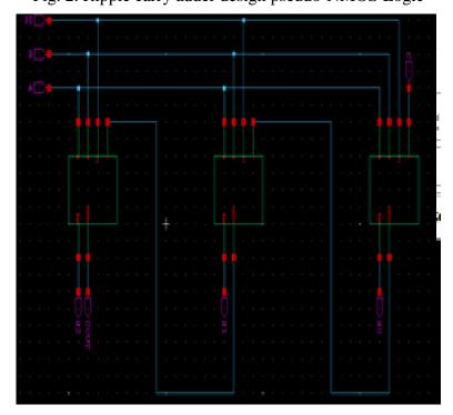
Fig. 3. Ripple carry adder design pseudo-NMOS Logic
