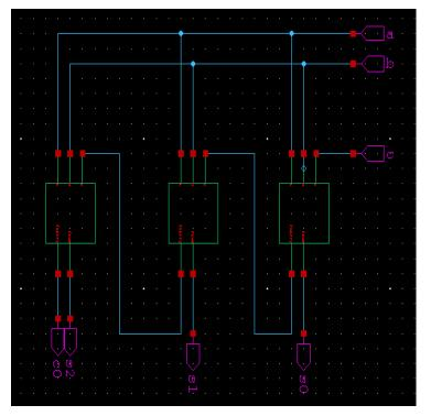
Fig. 2. Ripple carry adder design pseudo-NMOS Logic
