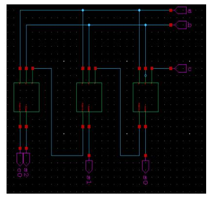
Fig. 4. Ripple carry adder design Pass transistor Logic
