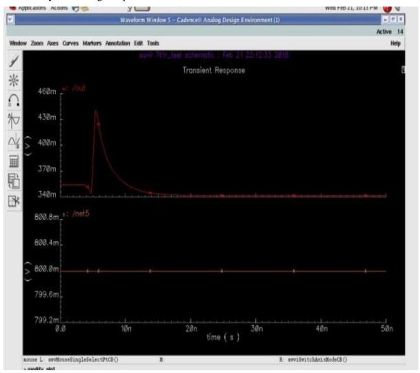
Figure 3. Simulation results of the proposed 7T SRAM cell
