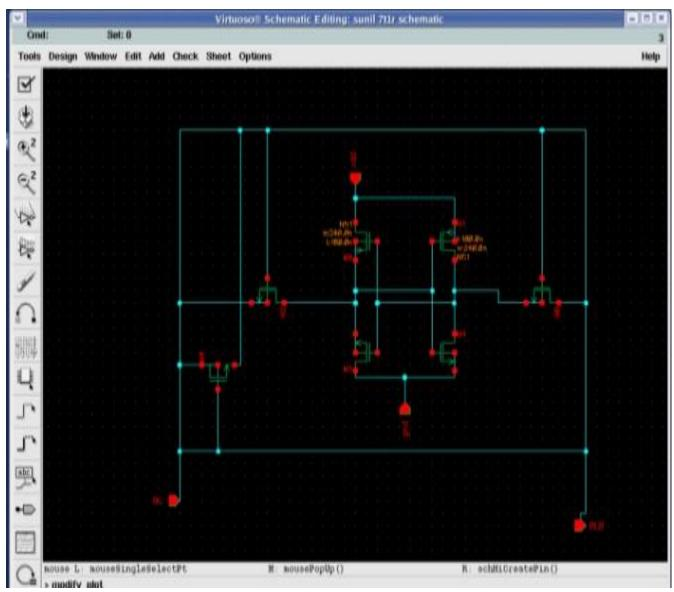
Figure 2. Scheme of the pproposed 7T SRAM cell design
