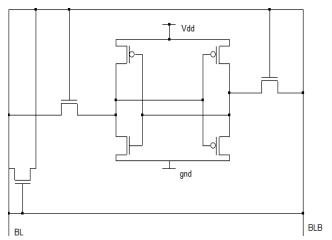
Figure 1. Proposed 7T SRAM cell
