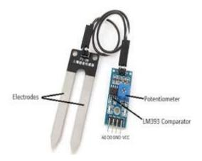
Fig. 3. Soil moisture sensor
