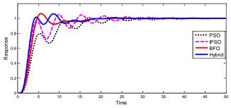
Fig. 10. Servo responses for Process 3 with optimized PID parameters
