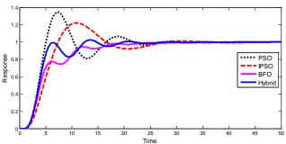
Fig. 8. Servo responses for Process 2 with soft computing based PID parameters (see online version for colours)
