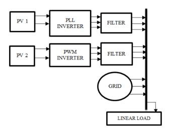
Fig. 5. Block diagram of linear load connected grid system
