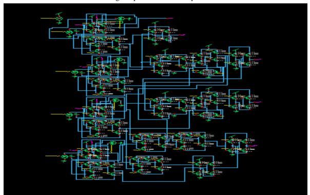
Fig. 2. Schematic of Pipelined Han Carlson Adder
