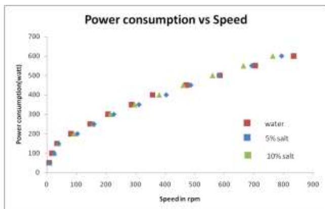
Fig. 5. Effect of impeller speed on power consumption for 30 cm liquid level.
