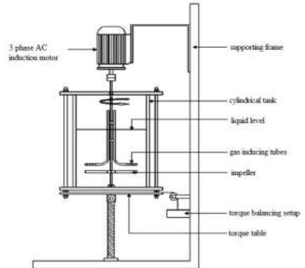
Fig. 1. Experimental setup of the conventional baffled agitated vessel retrofitted with the proposed air-inducing impeller system
