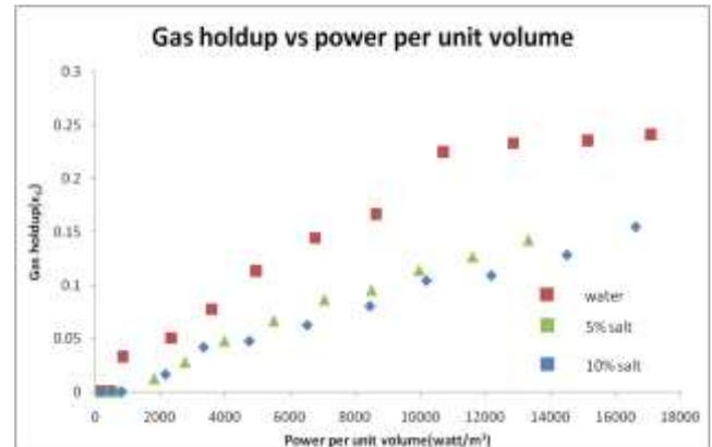
Fig. 3. Effect of concentration of NaCl in working fluid on gas holdup for 30 cm liquid level
