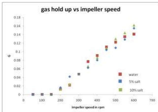
Fig. 4. Effect of impeller speed on fractional gas holdup ( $\epsilon$ ) for 30 cm liquid level
