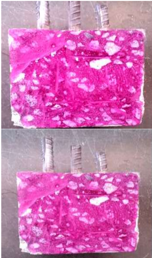
Figure 5. Phenolphthalein indicator sprayed in the fresh fracture Re-alkalized treated cut specimen
