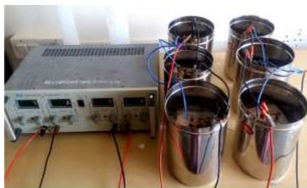
Figure 4. ER treatment for acid treated reinforced concrete cubes
