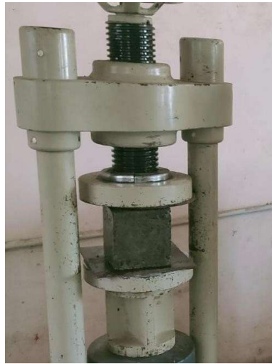
FIGURE 3. Compression Strength Testing of Cubes
