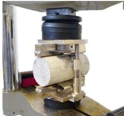
FIGURE 4. Split Tensile Strength Testing of Cylinders
