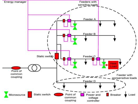
Fig. 1. Architecture of microgrid
