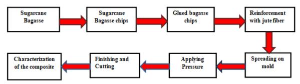
Figure 1. Processes to manufacture the composite
