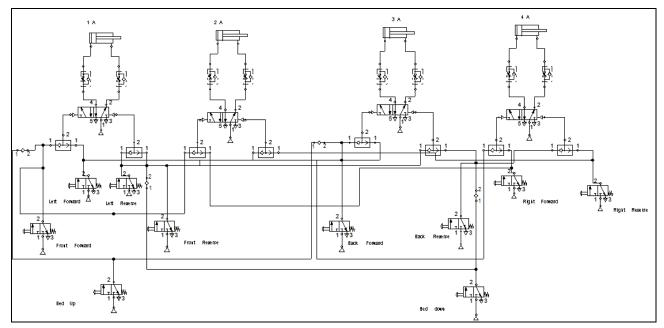
Figure 3. Pneumatic circuit in bed stable position
