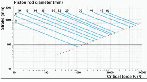
Figure 12. Stroke length, piston rod diameter and critical force relation diagram (Courtesy: Engineering Tool Box)
