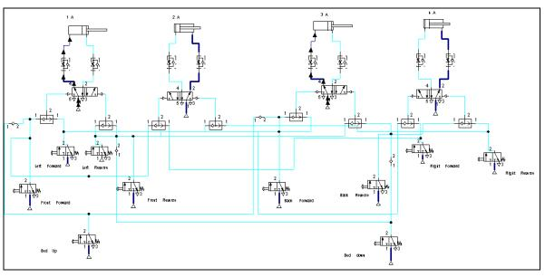
Figure 8. Pneumatic design for raise of bed
