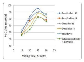
Figure 6. Percent of colour removal with mixing time in simple extract
