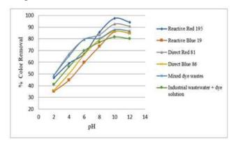
Figure 9. Effect of pH on colour removal under saline extract
