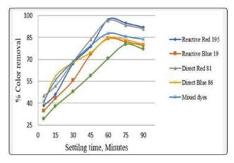
Figure 5. Percent of colour removal vs settling time for Saline extract
