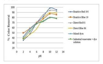
Figure 8. Effect of pH on colour removal under simple extract
