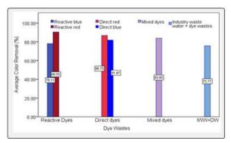
Figure 12. Effect of dye types on colour removal with moringa seed extract
