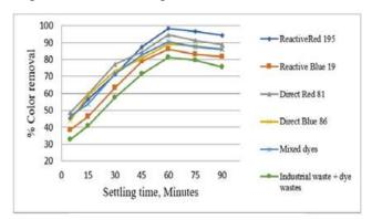
Figure 4. Percent of colour removal vs settling time for simple extract
